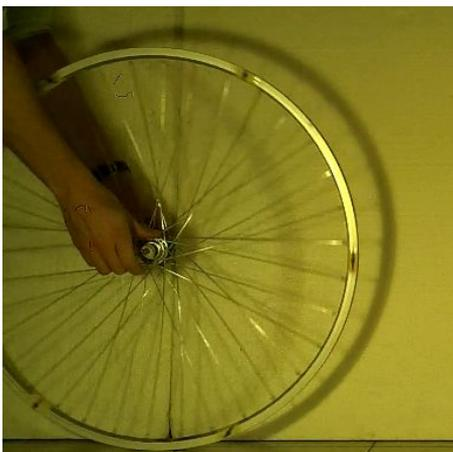
Figure 1. Experimental set-up: A rotating wheel was placed in contact with the floor. The centre of mass and a point located on the wheel rim were tracked and the displacement versus time data were analysed using
